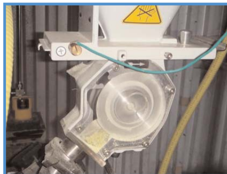
The Neundorfer-designed granular sulfur feeder is mechanically simple and is easy for operators to maintain.
